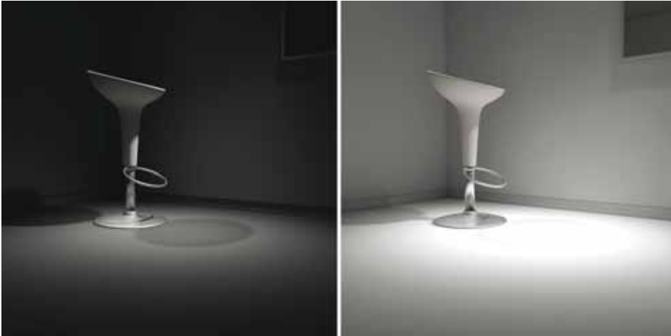
Figure 6-4. A dark floor vs. a pale floor under identical lighting conditions - nothing else has changed; the amount of reflected light (reflectance) has a direct relation with the material color (and vice versa).
